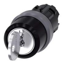
RONIS key-operated switch, 22 mm, round, plastic with metal front ring, lock number SB30, with 2 keys, 3 switch positions I>O<II, momentary contact on the left, latching on the right, actuating angle 2x45°, 10:30h/12h/13:30h, Key removal II, possible special locks: SB31, 421, 455, with laser labeling, inscription or symbol Customer-specific selection with SIRIUS ACT configurator (CIN)
