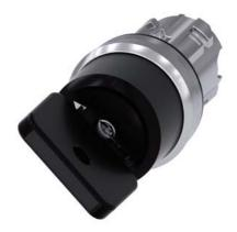
Key-operated switch O.M.R, 22 mm, round, metal, shiny, lock number 73034, black, with 2 keys, 2 switch positions O-I, latching, actuating angle  $90^{\circ}$ , 10:30h/13:30h, key removal I, with laser labeling, lower case
