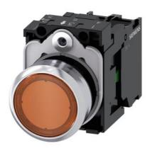
Illuminated pushbutton, 22 mm, round, metal, shiny, amber, pushbutton, flat, momentary contact type, with holder, 1NO, LED module with integrated LED 230 V AC, screw terminal, with laser labeling, inscription or symbol Customer-specific selection with SIRIUS ACT configurator (CIN)
