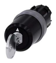
Key-operated switch BKS, 22 mm, round, plastic with metal front ring, lock number S1, with 2 keys, 3 switch positions I-O-II, latching, actuating angle 2x45°, 10:30h/12h/13:30h, Key removal I+O+II, Z=50-unit packaging
