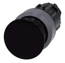
Mushroom pushbutton, 22 mm, round, plastic with metal front ring, black, 30 mm, momentary contact type, with laser labeling, symbol number according to, ISO 7000 or IEC 60417
