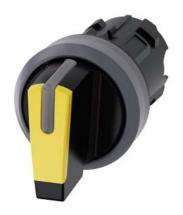
Selector switch, illuminable, 22 mm, round, plastic with metal front ring, yellow, selector switch, short, 3 switch positions I>O<II, momentary contact type, actuating angle 2x45°, 10:30h/12h/13:30h, with laser labeling, upper case and lower case, always upper case at beginning of line
