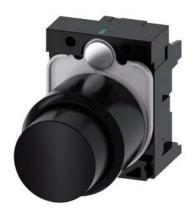
Pushbutton, compact, with extended stroke (12 mm), 22 mm, round, plastic, black, pushbutton, high, momentary contact type, with holder, with laser labeling, upper case and lower case, always upper case at beginning of line
