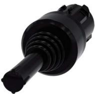
Coordinate switch, 22 mm, round, plastic, black, 2 switch positions, horizontal latching, without mechanical interlocking, with laser labeling, inscription or symbol, Customer-specific selection with SIRIUS ACT configurator (CIN)
