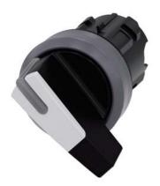
Selector switch, illuminable, 22 mm, round, plastic with metal front ring, white, selector switch, long, 2 switch positions O-I, latching, actuating angle  $90^{\circ}$ , 10:30h/13:30h, with laser labeling, lower case
