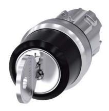
RONIS key-operated switch, 22 mm, round, metal, shiny, lock number SB30, with 2 keys, 3 switch positions I-O-II, latching, actuating angle 2x45°, 10:30h/12h/13:30h, Key removal I+II, possible special locks: SB31, 421, 455, with laser labeling, upper case and lower case, always upper case at beginning of line
