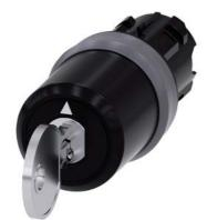
key-operated switch Siemens, 22 mm, round, plastic with metal front ring, lock number SSG10, with 2 keys, 3 switch positions I-O-II, latching, actuating angle  $2x45^{\circ}$ , 10:30h/12h/13:30h, key removal I+O+II, with laser labeling, upper case and lower case, always upper case at the beginning of the word
