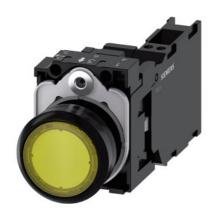
Illuminated pushbutton, 22 mm, round, plastic, yellow, pushbutton, flat, momentary contact type, with holder, 1 NO+1 NC, LED module with integrated LED 24 V AC/DC, spring-type terminal, Z=20-unit packaging
