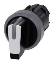
Selector switch, illuminable, 22 mm, round, plastic with metal front ring, white, selector switch, short, 3 switch positions I>O<II, momentary contact type, actuating angle 2x45°, 10:30h/12h/13:30h, with laser labeling, inscription or symbol Customer-specific selection with SIRIUS ACT configurator (CIN)
