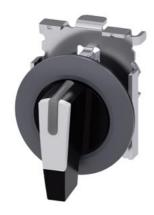
Selector switch, illuminable, 30 mm, round, Metal, matte, white, selector switch, long, front ring for flush installation, 3 switch positions I>O<II, momentary contact type, actuating angle 2x45°, 10:30h/12h/13:30h, with laser labeling, lower case
