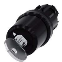
key-operated switch Siemens, 22 mm, round, plastic, lock number SSG10, with 2 keys, 2 switch positions O-I, latching, actuating angle 90°, 10:30h/13:30h, key removal O, with laser labeling, upper case and lower case, always upper case at the beginning of the word
