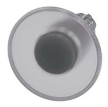
Illuminated mushroom pushbutton, 22 mm, round, metal, shiny, clear, 60 mm, latching, pull-to-unlatch mechanism, with laser labeling, symbol number according to, ISO 7000 or IEC 60417
