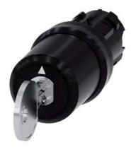
key-operated switch Siemens, 22 mm, round, plastic, lock number SSG10, with 2 keys, 3 switch positions I>O<II, momentary contact on the left, latching on the right, actuating angle 2x45°, 10:30h/12h/13:30h, key removal O, with laser labeling, inscription or symbol customer-specific selection with SIRIUS ACT configurator (CIN)
