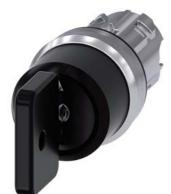
Key-operated switch O.M.R, 22 mm, round, metal, shiny, lock number 73034, black, with 2 keys, 3 switch positions I-O-II, latching, actuating angle 2x45°, 10:30h/12h/13:30h, Key removal I+O+II, with laser labeling, inscription or symbol Customer-specific selection with SIRIUS ACT configurator (CIN)
