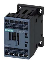
Power contactor, AC-3 16 A, 7.5 kW / 400 V 1 NC, 220 V AC, 50/60 Hz 3-pole, Size S00 Spring-type terminals
