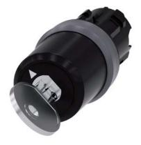
Key-operated switch BKS, 22 mm, round, plastic with metal front ring, Lock No. E9 (VW), without key, 2 switch positions O-I, latching, actuating angle  $90^{\circ}$ , 10:30h/13:30h, Key removal O+I
