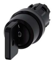
Key-operated switch O.M.R, 22 mm, round, plastic, lock number 73034, black, with 2 keys, 3 switch positions I>O<II, momentary contact type, actuating angle  $2x45^{\circ}$ , 10:30h/12h/13:30h, key removal O, with laser labeling, upper case and lower case, always upper case at the beginning of the word
