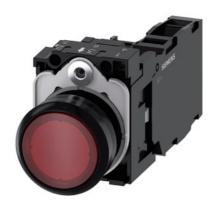
Illuminated pushbutton, 22 mm, round, plastic, red, pushbutton, flat, momentary contact type, with holder, 1 NO+1 NC, LED module with integrated LED 110 V AC, screw terminal, with laser labeling, inscription or symbol Customer-specific selection with SIRIUS ACT configurator (CIN)
