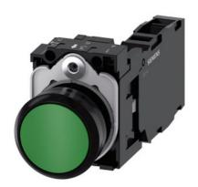
Pushbutton, 22 mm, round, plastic, green, pushbutton, flat, momentary contact type, with holder 1 NO+1 NC, screw terminal, with laser labeling, lower case
