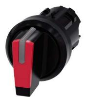
Selector switch, illuminable, 22 mm, round, plastic, red, selector switch, short, 3 switch positions I>O<II, momentary contact type, actuating angle 2x45°, 10:30h/12h/13:30h, with laser labeling, lower case
