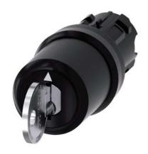
Key-operated switch IKON, 22 mm, round, plastic, lock number 360012K1, with 2 keys, 3 switch positions I-O-II, latching, actuating angle 2x45°, 10:30h/12h/13:30h, key removal O, with laser labeling, upper case and lower case, always upper case at beginning of line
