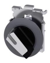
Selector switch, illuminable, 30 mm, round, Metal, matte, white, selector switch, short, front ring for flush installation, 2 switch positions O-I, latching, actuating angle 90°, 10:30h/13:30h, Z=50-unit packaging
