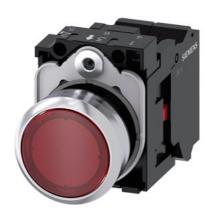
Illuminated pushbutton, 22 mm, round, metal, shiny, red, pushbutton, flat, momentary contact type, with holder, 1NC, LED module with integrated LED 110 V AC, spring-type terminal, with laser labeling, lower case
