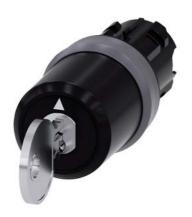
key-operated switch Siemens, 22 mm, round, plastic with metal front ring, lock number SSG10, with 2 keys, 3 switch positions I>O<II, momentary contact on the left, latching on the right, actuating angle  $2x45^{\circ}, 10:30h/12h/13:30h,$  key removal O Z=50-unit packaging
