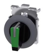
Selector switch, illuminable, 30 mm, round, Metal, matte, green, selector switch, short, front ring for flush installation, 3 switch positions I>O<II, momentary contact type, actuating angle 2x45°, 10:30h/12h/13:30h, with laser labeling, upper case
