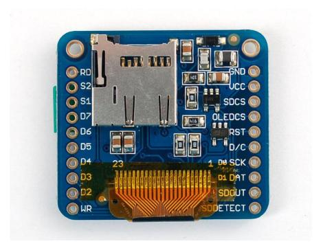
We'll have to add an extra 2 wires so we can 'select' and 'receive data' from the SD card
