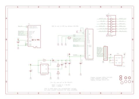
For the level shifter we use the  $\underline{CD74HC4050}$  () which has a typical propagation delay of ~10ns
