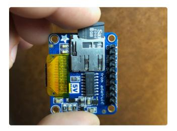
Insert the card Insert the micro SD card into the slot on the back of the SSD1331 breakout board.
