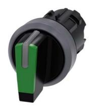
Selector switch, illuminable, 22 mm, round, plastic with metal front ring, green, selector switch, short, 3 switch positions I-O<II, left latching, right momentary contact type, actuating angle 2x45°, 10:30h/12h/13:30h, with laser labeling, lower case
