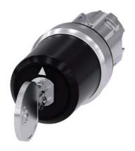
Key-operated switch BKS, 22 mm, round, metal, shiny, lock number S1, with 2 keys, 3 switch positions I-O-II, latching, actuating angle  $2x45^{\circ}$ , 10:30h/12h/13:30h, Key removal I+O+II, Z=50-unit packaging
