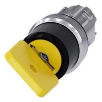
Key-operated switch O.M.R, 22 mm, round, metal, shiny, lock number 73033, yellow, with 2 keys, 2 switch positions O<I, momentary contact type, Actuating angle 45°, 10:30h/12h, key removal O, with laser labeling, upper case
