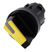
Selector switch, illuminable, 22 mm, round, plastic, yellow, selector switch, short, 2 switch positions O-I, latching, actuating angle  $90^\circ$ , 10:30h/13:30h Z=50-unit packaging
