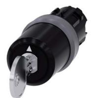
Key-operated switch BKS, 22 mm, round, plastic with metal front ring, lock number S1, with 2 keys, 3 switch positions I-O-II, latching, actuating angle  $2x45^{\circ}$ , 10:30h/12h/13:30h, Key removal II, with laser labeling, lower case
