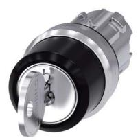
RONIS key-operated switch, 22 mm, round, metal, shiny, lock number SB30, with 2 keys, 3 switch positions I>O<II, momentary contact type, actuating angle 2x45°, 10:30h/12h/13:30h, key removal O, possible special locks: SB31, 421, 455, with laser labeling, inscription or symbol Customer-specific selection with SIRIUS ACT configurator (CIN)
