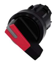
Selector switch, illuminable, 22 mm, round, plastic, red, selector switch, long, 2 switch positions O-I, latching, actuating angle 90°, 10:30h/13:30h, with laser labeling, upper case and lower case, always upper case at the beginning of the word
