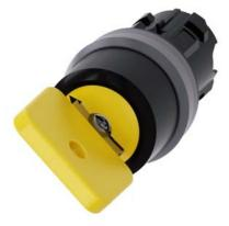
Key-operated switch O.M.R, 22 mm, round, plastic with metal front ring, lock number 73033, yellow, with 2 keys, 2 switch positions O-I, latching, actuating angle 90°, 10:30h/13:30h, key removal O+I, Z=50-unit packaging
