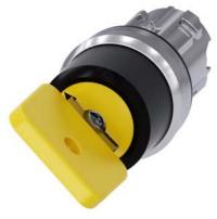
Key-operated switch O.M.R, 22 mm, round, metal, shiny, lock number 73033, yellow, with 2 keys, 2 switch positions O<I, momentary contact type, Actuating angle 45°, 10:30h/12h, key removal O, with laser labeling, lower case
