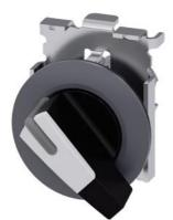
Selector switch, illuminable, 30 mm, round, Metal, matte, white, selector switch, long, front ring for flush installation, 2 switch positions O-I, latching, actuating angle 90°, 10:30h/13:30h, with laser labeling, upper case and lower case, always upper case at beginning of line
