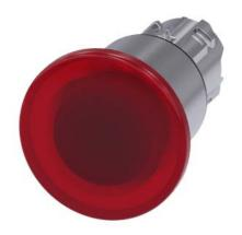
Illuminated mushroom pushbutton, 22 mm, round, metal, shiny, red, 40 mm, 3 switch positions, latches after pushing in, unlatches by pull-to-unlatch mechanism to center position, after pulling out the button Retraction to center position, with laser labeling, lower case
