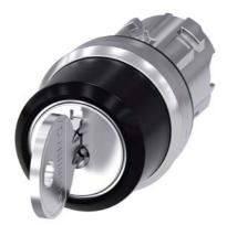
RONIS key-operated switch, 22 mm, round, metal, shiny, lock number SB30, with 2 keys, 3 switch positions I-O-II, latching, actuating angle 2x45°, 10:30h/12h/13:30h, Key removal II, possible special locks: SB31, 421, 455, with laser labeling, lower case
