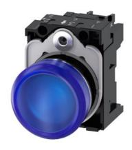
Indicator lights, 22 mm, round, metal, shiny, blue, lens, smooth, with holder, LED module with integrated LED 24 V AC/DC, screw terminal, with laser labeling, upper case and lower case, always upper case at the beginning of the word
