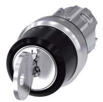
RONIS key-operated switch, 22 mm, round, metal, shiny, lock number SB30, with 2 keys, 3 switch positions I>O<II, momentary contact on the left, latching on the right, actuating angle 2x45°, 10:30h/12h/13:30h, key removal O, possible special locks: SB31, 421, 455, with laser labeling, upper case
