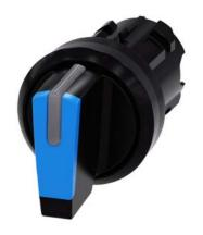
Selector switch, illuminable, 22 mm, round, plastic, blue, selector switch, short, 3 switch positions I-O<II, left latching, right momentary contact type, actuating angle  $2x45^{\circ}$ , 10:30h/12h/13:30h, with laser labeling, upper case and lower case, always upper case at the beginning of the word
