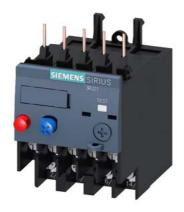
Overload relay 0.35...0.50 A Thermal For motor protection Size S00, Class 10 Contactor mounting Main circuit: Ring cable lug Auxiliary circuit: ring cable lug Manual-Automatic-Reset
