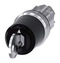
Key-operated switch IKON, 22 mm, round, metal, shiny, lock number 360012K1, with 2 keys, 3 switch positions I-O-II, latching, actuating angle 2x45°, 10:30h/12h/13:30h, key removal O, with laser labeling, upper case and lower case, always upper case at beginning of line
