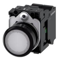
Illuminated pushbutton, 22 mm, round, plastic, white, pushbutton, flat, momentary contact type, with holder, 1NO, LED module with integrated LED 24 V AC/DC, spring-type terminal, with laser labeling, lower case
