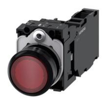
Illuminated pushbutton, 22 mm, round, plastic, red, pushbutton, flat, momentary contact type, with holder, 1 NO+1 NC, LED module with integrated LED 24 V AC/DC, screw terminal, with laser labeling, upper case and lower case, Always upper case at the beginning of the word
