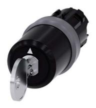
key-operated switch Siemens, 22 mm, round, plastic with metal front ring, lock number SSG10, with 2 keys, 3 switch positions I-O-II, latching, actuating angle 2x45°, 10:30h/12h/13:30h, key removal I+II, with laser labeling, upper case and lower case, always upper case at beginning of line
